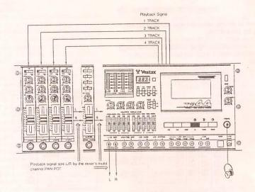
The above is the connecting structure of each section of MR-44. For further information, please refer to the block diagram in the last page. It is emphasised that of if you can
